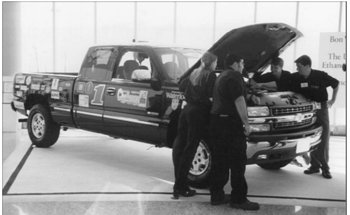
This 1999 Chevy Silverado 5.3L Vortec V8 Extended Cab 4x4 Pickup truck was re-engineered from a dedicated gasoline power to dedicated fuel ethanol power.
