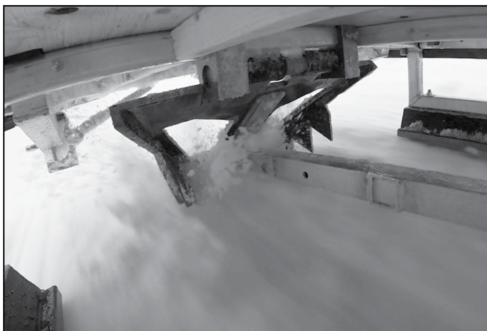
University of Waterloo Concrete Toboggan Team The toboggan’s braking mechanism.
