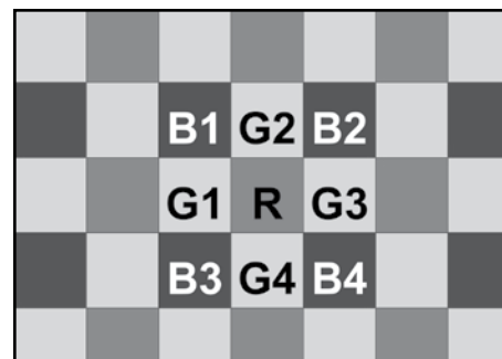
Typical bayer pattern colour filter arrangement of an image sensor
