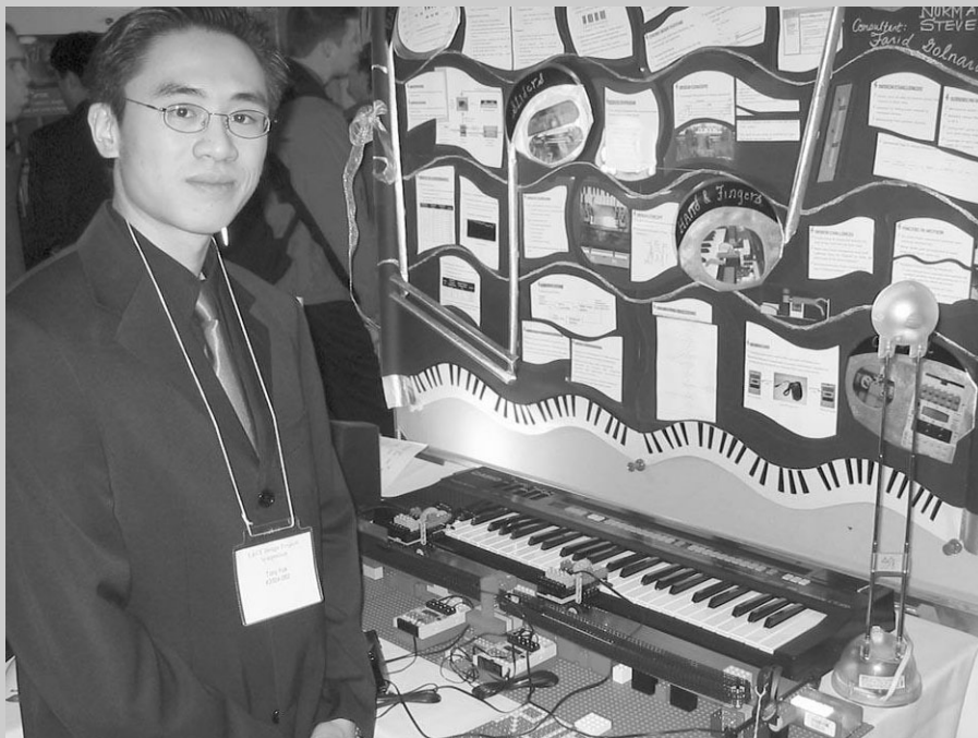
The Robotic Pianist mimics the human piano-playing gesture with a pair of robotic hands that have the capability of automatically playing simple music pieces.
