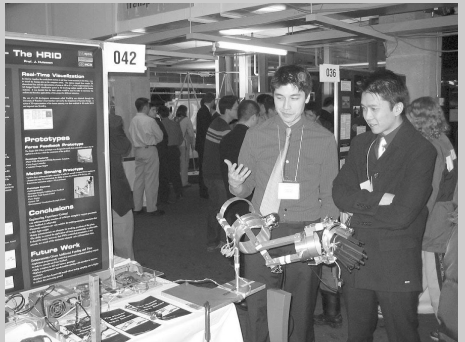
This human-machine interface combines the ability to sense the complete range of human motion and provides sensory feedback to the operator.
